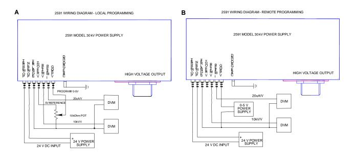
Fig. 3. Local (A) and remote (B) programming connections
