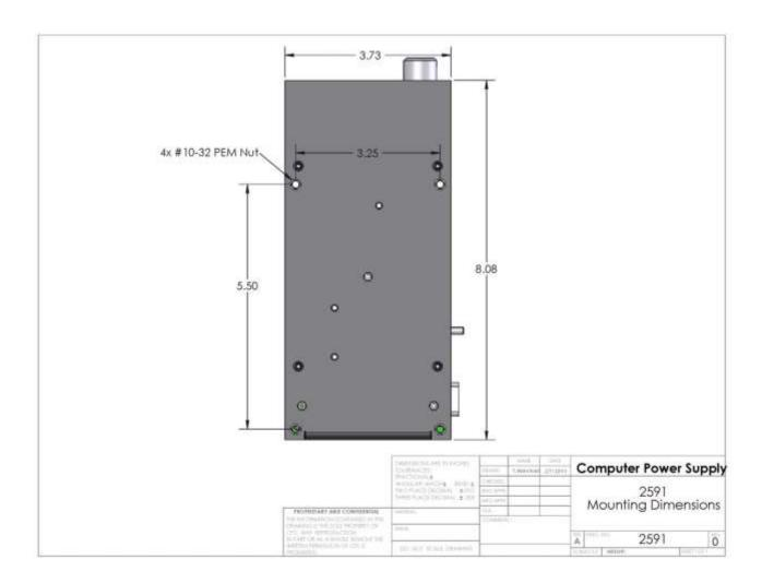
Fig. 2. Physical layout showing the placement of mounting holes on the bottom panel of 2591 power supply.
