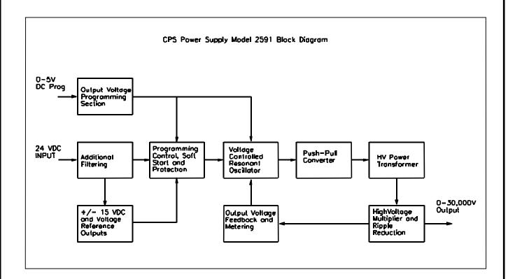
Fig. 1. Block diagram of 2591 high voltage power supply
