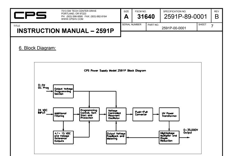
Fig. 1. Block diagram of 2591P high voltage power supply
