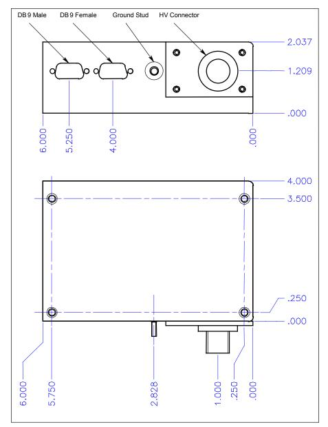
Fig. 2. Physical layout showing the placement of mounting holes on the bottom panel of 2591P power supply
