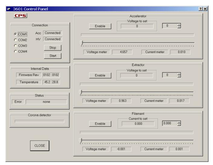
Figure 4. Control Panel screen.
