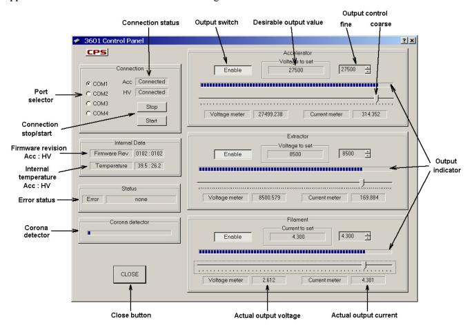
Figure 5. Control Panel screen.
