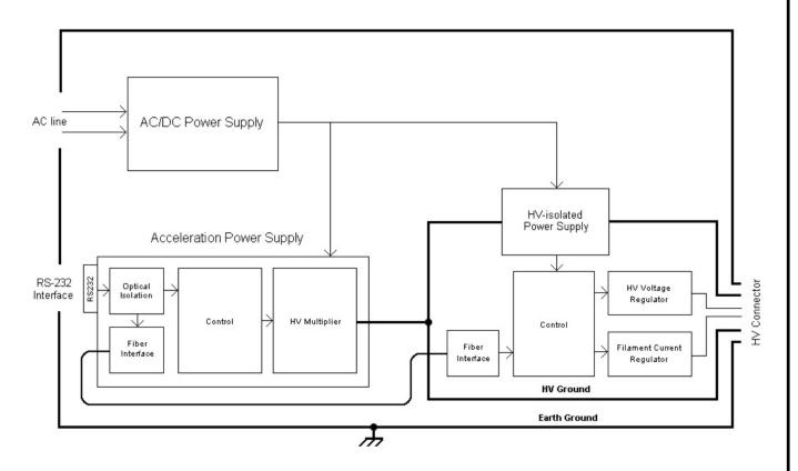
Figure 1. Block Diagram of 3601.
